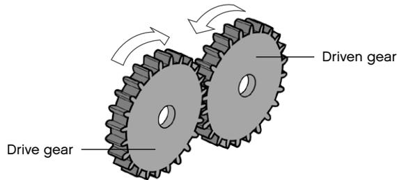
The drive gear is the gear that is turned by an outside effort, for instance your hand or an engine. Any gear that is turned by another gear is called a driven gear. The drive gear provides the input force and the driven gear delivers the output force.
